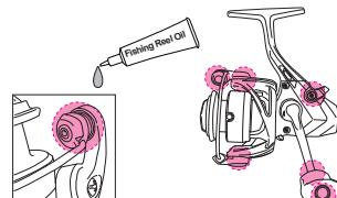
\* Apply reel oil to the highlighted parts in diagram above.
