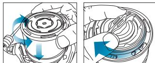
Slide spool onto the main shaft and turn the drag knob clockwise to tighten and increase drag pressure.
