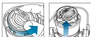
Turn the drag knob counterclockwise to loosen and pull the spool off the spool shaft.
